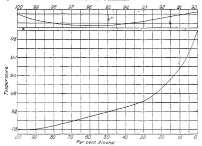
alcohol by distillation to a strength of 30 or 40 per cent. by weight, while the further concentration is relatively difficult.
